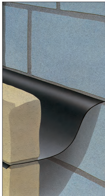
Detail showing built in cavity tray
