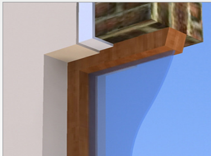
WRB laminate in position
