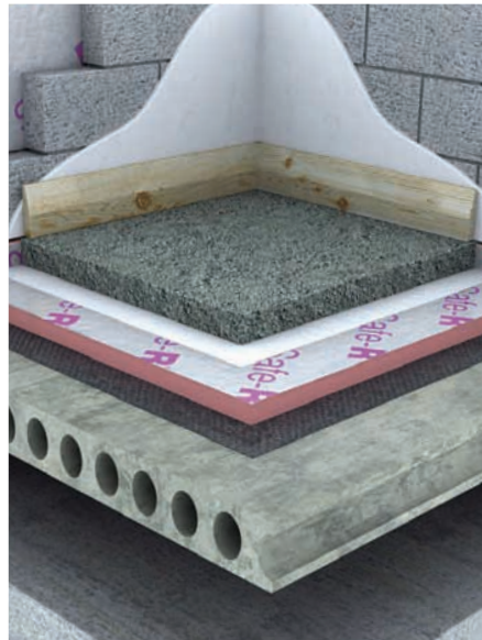
Safe-R Layed Below Concrete Floor Screed
