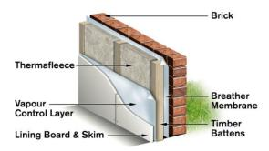
Fit a breather membrane to the inner face of the solid wall on the cold side of the insulation and fit a vapour control layer to the warm side before installing the wall finishing.
