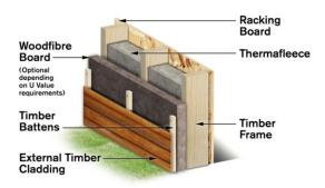
Unlike traditional timber frame systems, the racking board is positioned to the inside of the timber frame. The external insulation attached to the timber frame maintains the frame above the dewpoint temperature reducing the risk of condensation. Additional benefits include low environmental impact, lightweight structure and improved insulation and airtightness.
