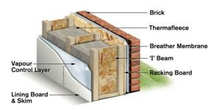
A service void can be created by counter battening along the timber frame internal face and fixing the internal finishing board. This ensures that the insulation remains undisturbed and airtightness remains intact when services are accessed for maintenance. The insulation performance of the void can be improved by installing an Eden Low Emissivity Membrane against the insulation.
