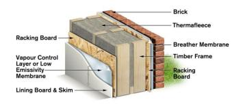
The twin frame system ensures that reduced thermal bridging occurs within the construction helping maximise insulation performance. By using two 89mm structural timber frames, the width of the construction can be varied to achieve specific insulation performance.
