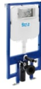
DUPLO WC COMPACT - Concealed floor standing structure with compact cistern (8 cm) and dual flush (4/2 - 4.5/3 - 6/3 L). 90 ø elbow.
