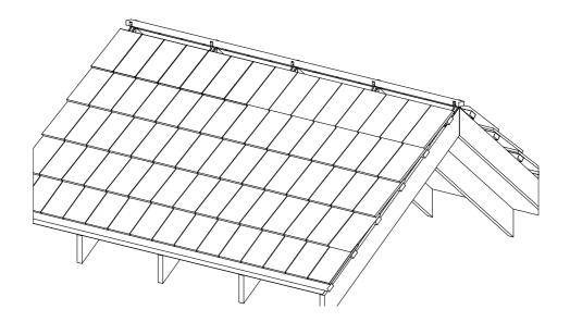
Ensure the top course of tiles is clean and dry. Then, unroll the ridge ventilation roll over the whole roof ridge. Use felt nails or staples to tack it to the ridge batten at 1-metre intervals.
