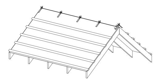
Lay timber batten between brackets. Make sure it overhangs the edge by 30mm at both ends. Fix the batten in place by nailing through the bracket into the top of the baton. Using 30mm stainless steel annular ring shanked nails (not supplied).
