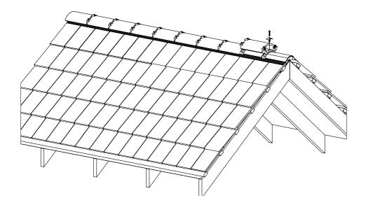
Any end ridge tiles should be fixed firmly in two places. It may be necessary to drill an additional hole to do this. Check that all tiles are securely attached.
