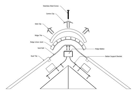
Lay the roofing underlay as per the latest BS5534 guidelines, matching the location and batten gauge. If ventilation is required, leave a gap before the apex of 5-8mm.
