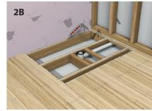
**2A.** Fit extra timbers where required to support edge of floor, tray and around trap. Screw existing floor to any new edge timbers. **2B.** Run a bead of **MEGA** Strength adhesive along the top of all joists and noggins. Stick the tray into position.
