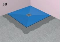
**3A.** Prime the concrete, then stick the tray down using a 4mm bed of flexible tile adhesive, ensuring that the top of the tray is flush with the existing floor level and that a 3mm gap is left between tray and walls. **3B.** Assemble and install the trap. Fill void around the tray with screed.
