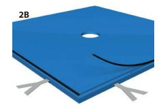
**2A.** Drill two 4mm holes into the outside edges of the tray and carefully screw in the four stainless steel anchors. **2B.** Stick the temporary 6mm rubber strip into the rebate of the room-facing edges of the tray.
