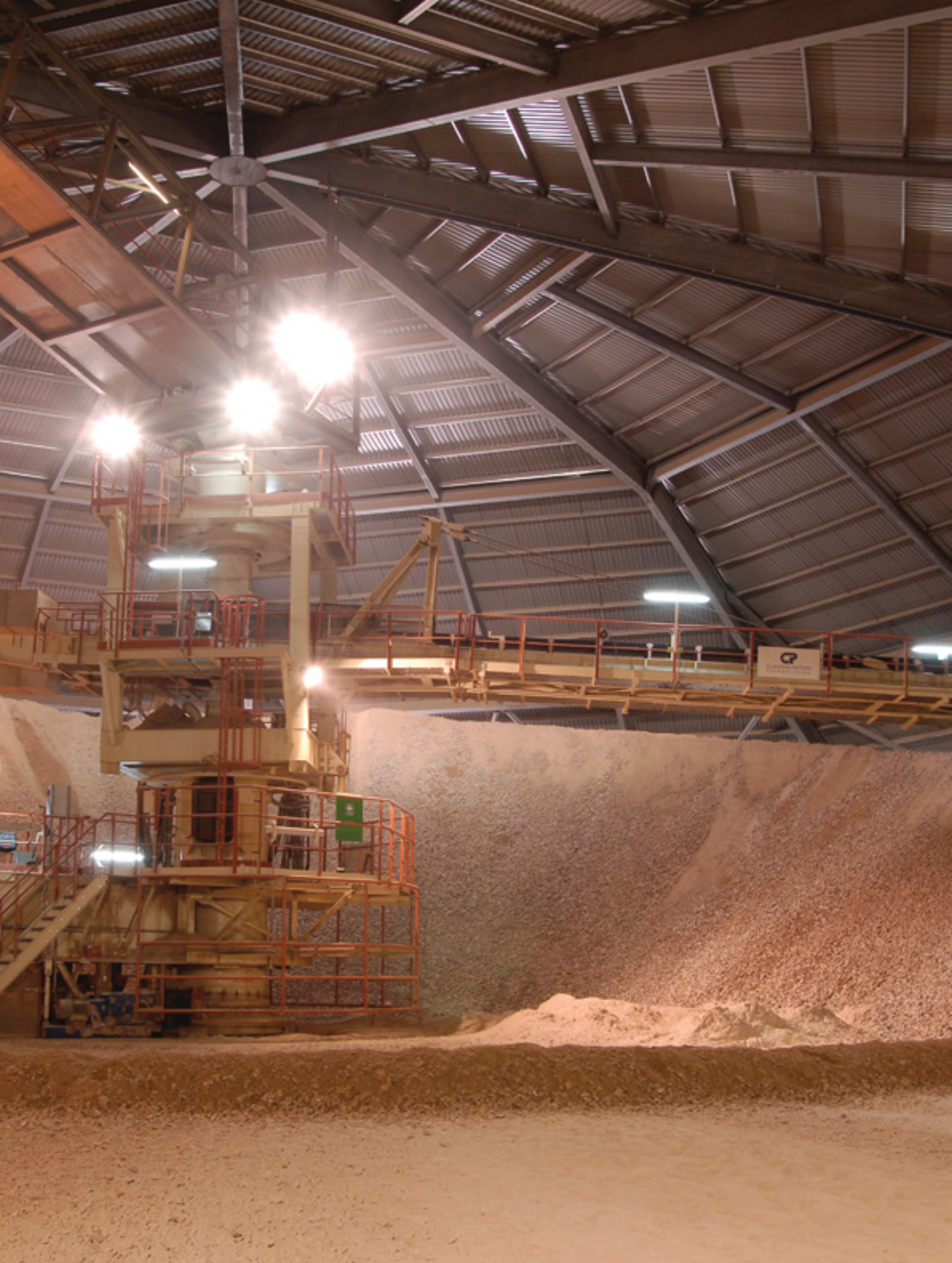
Homogeniser, Barrow-upon-Soar, Leicestershire, where mined gypsum is stored
