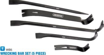
Set comprising of two pry bars, two wrecking bars and an aligning bar. All bars are manufactured from high grade steel hardened at both ends. Display packed Contents: • Pry bar (180mm) • Pry bar (350mm) • Aligning bar (450mm) • Wrecking bar (300mm) • Wrecking bar (450mm)
