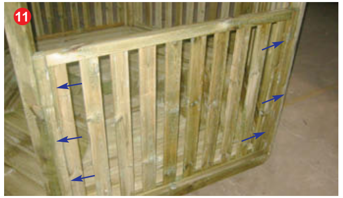
Sit the large fence on the floor between the uprights and secure with 6 x 70mm screws. It may help to drill pilot holes in the end frames of all the fence.
