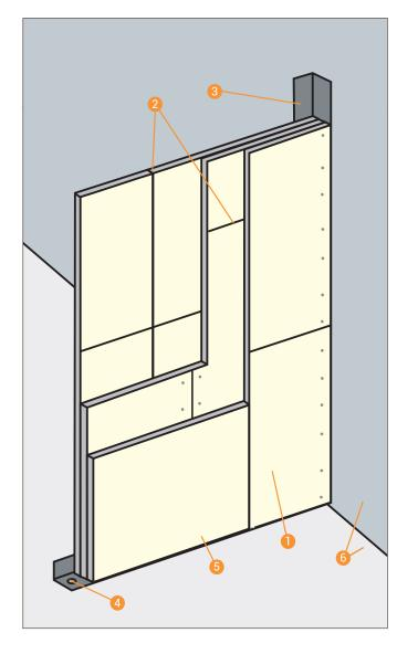
Solid Partitions EI 30 to EI 240 Integrity and Insulation in both directions
