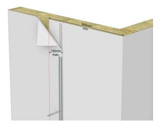
Figure 2 - External corner arrangement
