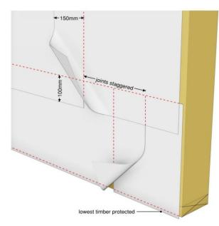
Figure 1 - Joint arrangement
