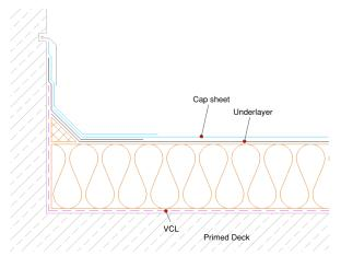
The vapour control layer (VCL) should be set out to facilitate a minimum 50mm link with the waterproofing layers, with completed detailing encapsulating the insulation. At all skirtings and upstands, the waterproofing should be at least 150mm above the level of the <u>finished</u> roof level. Care must be undertaken not to bridge over any DPC or Cavity Tray positions.
