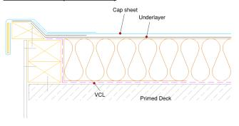
Check kerbs should be constructed to form a 50mm water check to prevent water from running over the edge incorporating a welted drip detail. The vapour control layer (VCL) should be set out to facilitate a minimum 50mm link with the waterproofing layers, with completed detailing encapsulating the insulation.
