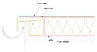
A welted drip edge should be formed wherever drainage to an external guttering is required. The vapour control layer (VCL) should be set out to facilitate a minimum 50mm link with the waterproofing layers, with completed detailing encapsulating the insulation. A plywood former should be introduced to form the drip. In warm roof build ups an insulated hard edge, 10mm thinner than the insulation thickness, should be incorporated.
