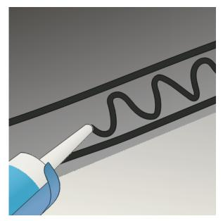
Figure 3 - Placing Lap Adhesive
