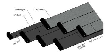
Figure 1 Setting Out to Staggered Laps
