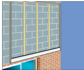
3. Fit first plank at base
