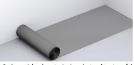
**2.** Spread the sheet in the lengthwise direction of the boards.
