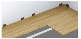
**4.** Install the floating wood floor according to the manufacturer's instructions.
