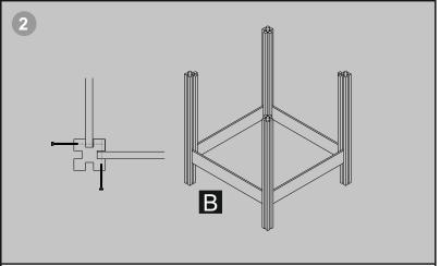
Slot the first row of boards into the framing. Secure 3 of the boards using the 50mm screws, 2 at each end of each board. The one board you do not secure will be your access to the compost so position it in an accessible orientation.
