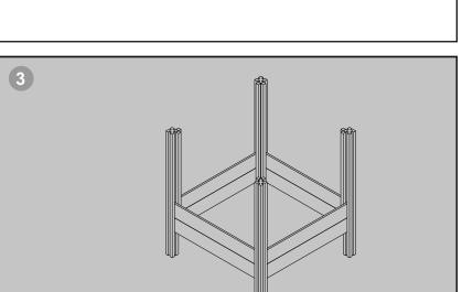
Slot the remainder of the boards into position. Secure all of the top boards using 2x50mm screws at each end of each board.
