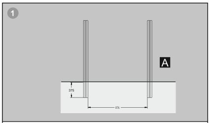
Position the posts in a square formation each post 923mm apart as shown and sink 375mm into the ground.
