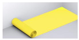
2. Extend the sheet in the longitudinal direction of the boards.
