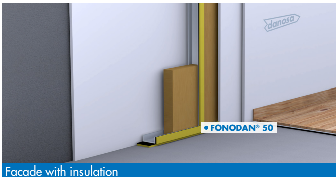
Facade with insulation
