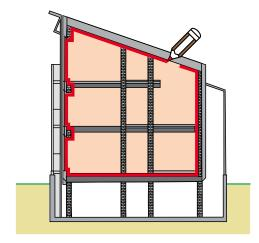
The main emphasis within the building element for the AT line is **INTERNALLY**. The component used for this would normally be the AVCL - behind the dry-lining. This membrane also has the important function of providing condensation control within the construction, by limiting vapour drive. To help with appropriate material selection. Please see the Products Application Chart.
