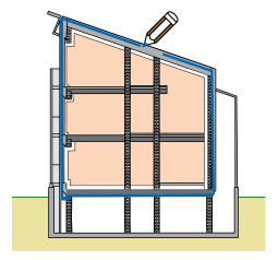
The AT line may also be established **EXTERNALLY**, on the cold side of the insulation. It is important that the layer being used for this is vapour-open to avoid trapped moisture within the element. A breather membrane with suitable resistance to air permeability would be ideal. Breather membranes with exceptional durability should be considered to give assurance of long-term performance.
