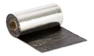
Self-adhesive Tape SELF-DAN 10 cm is a waterproofing bituminous tape, 10 cm wide, with metallic self-protection ( $1.2 \text{ kg/m}^2$ ). Composed of a SBS modified bitumen mastic, using as protective material on the upper side of the sheet aluminium foil (60 micron) in natural colour. The anti-adherent material used on the lower side is polyethylene film. Used for small leaks, chimneys, in carpentry, etc.
