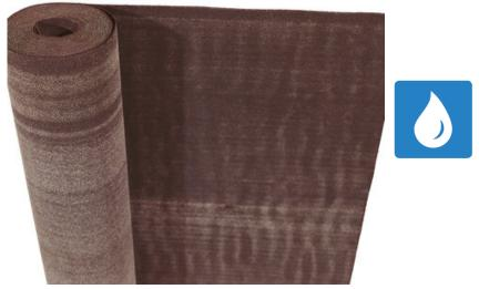
IMPERDAN FP 3 MM AP is a waterproofing bituminous sheet with sanded finishing, 3 mm thickness. Composed of a non-woven polyester felt reinforcement and covered on both sides with polymer modified bitumen (pliability -5°C) mastic. Membrane with an upper surface finish of sand and a lower surface finish of polyethylene film. Tested according to standard EN test methods.
