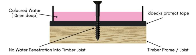
Completely Self Sealed When Fastener Is Driven Through The DDecks Protect Tape
