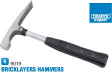
Expert Quality, polished and ground solid forged head and cutting edge from fine grain high carbon steel correctly hardened and tempered with a lacquer coating for rust protection. Hardened tubular shaft fitted with shock absorbing vinyl grip. Sold Loose.
