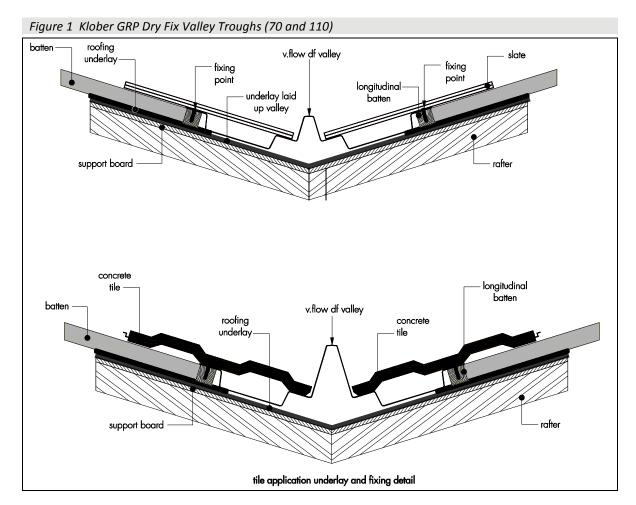
1.2 The profiles are supplied in lengths of 3 m, with widths of 400 mm and depths of either 70 or 110 mm.
