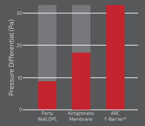
Results presented were obtained using a 100mm party wall cavity with a 100mm external cavity.
