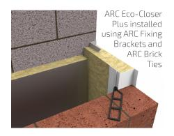
ARC Fixing Brackets should be used to mechanically fix Eco-Closer Plus to the inner blockwork, while ARC Brick Ties are then used to build the closer in as the external brickwork progresses. We recommend a minimum of 2 of each is used per metre, or piece, whichever is shorter.
