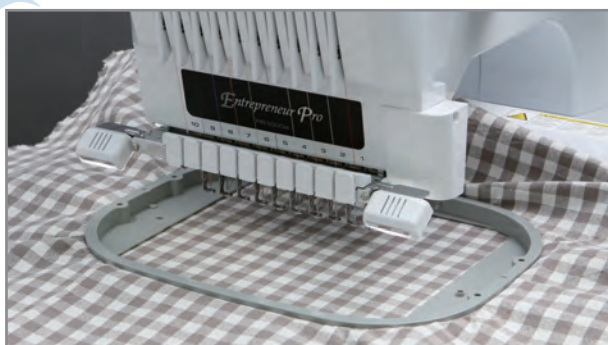
Square frame to make aligning quilt patterns and other embroidery positions easy
