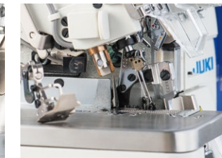
3. Presser foot arm with an open/close sensor
