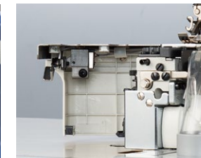
2. Cloth plate cover with an open/close microswitch
