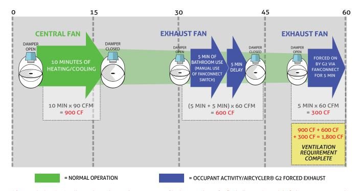
After regular heating/cooling cycles and manual occupant use of bathroom exhaust fan (including 5 minute delay), there was not enough ventilation to meet requirements for the hour. At the end of the hour the AirCycler® g2 forced on the bathroom exhaust fan, via the FanConnect™ switch, to reach required ventilation.
