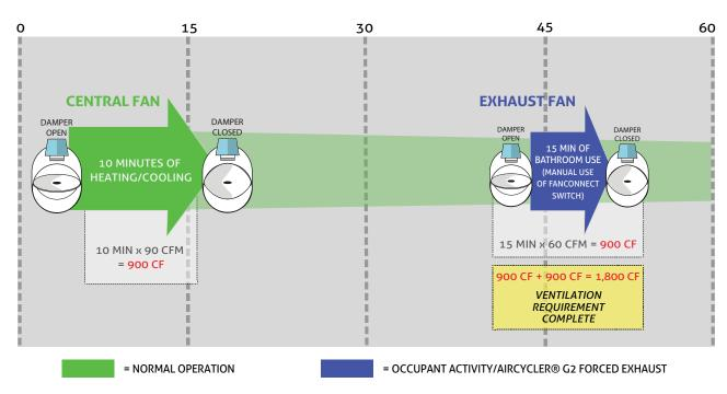
After regular heating/cooling cycles and manual occupant use of bathroom exhaust fan, ventilation requirements for the hour were met. No need for additional ventilation forced by AirCycler® g2.
