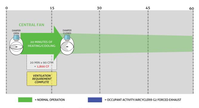
Enough ventilation took place during normal heating/cooling cycles to meet ventilation requirements for the hour.
