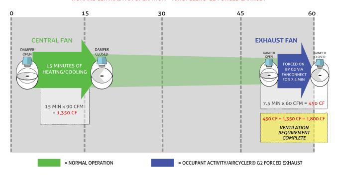
After regular heating/cooling cycles, ventilation requirements for the hour were not met. At the end of the hour the AirCycler® g2 forced on the bathroom exhaust fan, via the FanConnect™ switch, to reach required ventilation.
