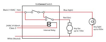
Inside the FanConnect™ switch is a 24VAC relay to control the 110VAC bath fan.
