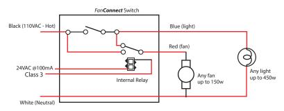
Inside the FanConnect™ switch is a 24VAC relay to control the 110VAC bath fan.
