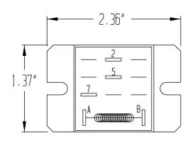
SPDT RELAY 120/240VAC 50-60Hz 1HP, 120VAC 30A, 1 1/2HP, 240VAC
