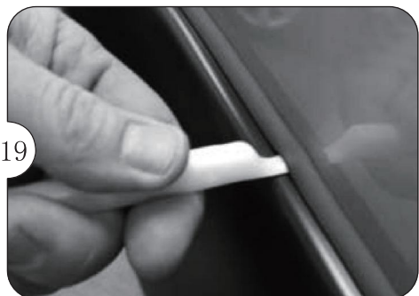
19 Using flat end of supplied Edge Trim Tool, seat edge trim against flare by inserting straight end between edge trim and flare at one end. Next, slide around entire edge to the other end.
