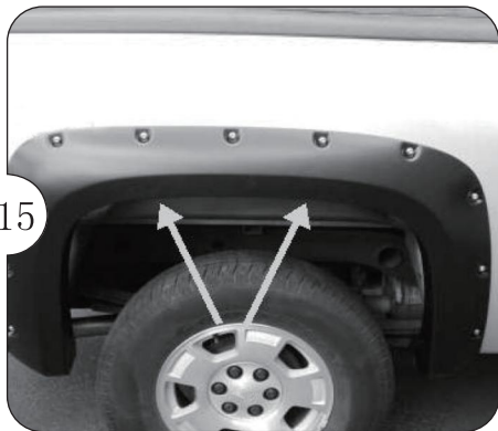
15 Reposition flare on fender. Start a supplied Screw through upper two hole locations and through each Clip installed in step 14. If needed, use awl to locate holes.
