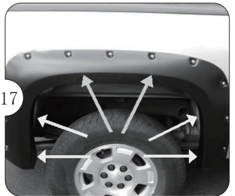
17 Fully tighten all screws starting with the newly installed Screws in upper two hole locations while pressing in on flare to ensure it is snug against sheet metal.
