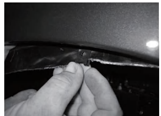
Photo #1 – Pull splash shield from behind fender. Install a supplied "U" Clip on splash shield as shown.
