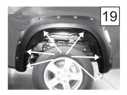
Hold flare firmly on the fender. Start a supplied Magni Black Screw through each hole in flare and into hole in fender. (6 locations)
