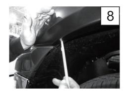
Hold front of the flare firmly on the fender. Mark three Spring Clip locations using the holes in the flare as a guide.
