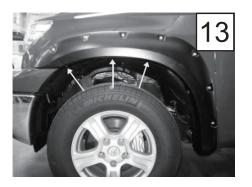
Start Phillips Truss Screw in location #1 first, then move to #2, and start in location #3 last.
