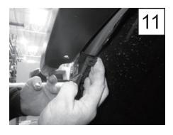
Slide a Spring Clip over each Mylar Tab.
