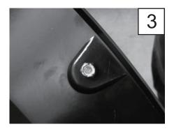
Place a Nylock Nut over the end of each Torx Screw and tighten, using a 1/2" wrench for the Nylock Nut and the supplied screw wrench for the Torx Screw. Repeat for remaining pockets.
