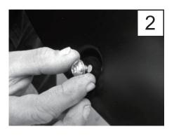
Put each Torx Screw through a pocket hole in the flare, screw head on the outside.
