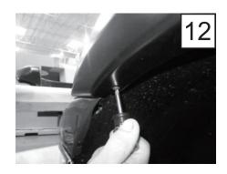
Align holes in flare with holes in Spring Clips. Start a supplied Phillips Truss Screw through holes in flare and into each Spring Clip installed in Step 11 in the order shown in Step 13. If necessary, use an awl to locate holes in clips.
