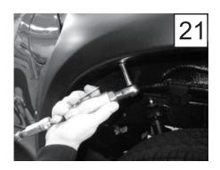
Ensure flare is properly positioned and tighten all screws.
