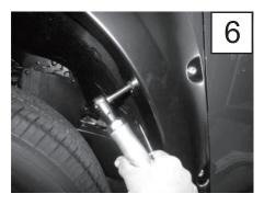
Start supplied Magni Black Screw through top rear hole in flare and into factory hole in rear of wheel well. Do not tighten.
