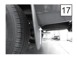
Remove one hex bolt from underside of mud flap using a 10mm socket.
