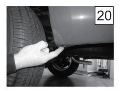
**NOTE:** If the lower rear wheel well does not contain a plastic grommet, insert supplied Screw Nylon Grommet into the factory hole as shown.
