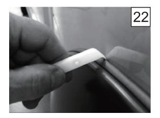
Using supplied Edge Trim Tool, seat edge trim against vehicle by hooking curved end under edge trim at one end of flare.
