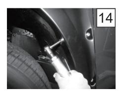
Start Magni Black Screw through the three lower rear holes in flare and into factory holes in rear of wheel well.
