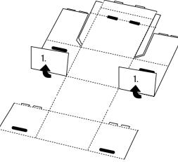
5 With flap (4) folded at a right angle, fold flap (3) inward. The tabs on flap (4) will allign with the grooves located on flap (1).
