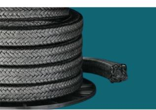
The graphited PTFE packing is braided from soft graphited PTFE yarn. This material is based on expanded, oriented fluorocarbon thin strips, which are incorporated with super fine flake graphite as a high temperature lubricant and an improver of a thermal conductivity.
