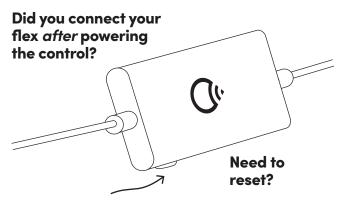
Press the button on the control in for 2–3 seconds. A light will run down the full length of the Neon Flex as it detects it. If it was connected before you plugged in the controller, it will automatically run this count.
