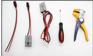
Materials needed before connecting solar panel with our battery that has Anderson Powerpole
