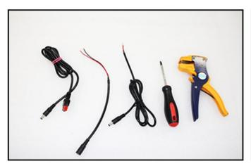
Materials needed before connecting solar panel with our line battery that has DC Barrel Plug and Anderson Powerpole.
