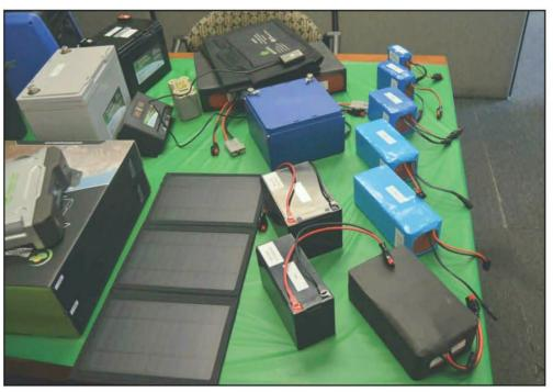
Photo A. Bioenno batteries include Lithium Iron Phosphate (LiFePO4) models that provide high current and high reliability with low weight.
