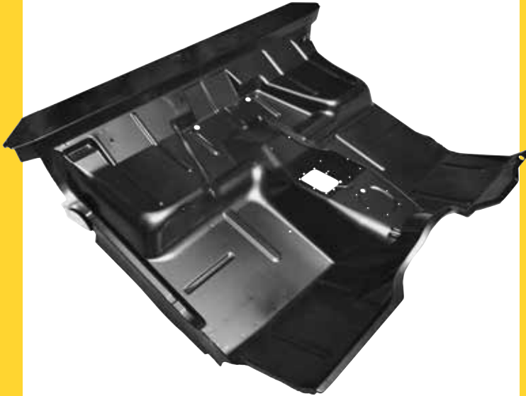
FP16-73 - Floor Panel Assembly 1973-87 Chevy/GMC Pickup, Higher Hump, without Removeable Trans Cover (4wd, Standard Cab)
