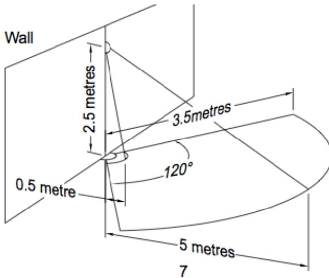
For optimal performance, your MultiSensor 6 should NOT be mounted directly on or near metal framing or other large metallic objects. Large metal objects may weaken the Z-Wave wireless signal MultiSensor 6 depends on for communication due to the wireless reflective properties of metal.
