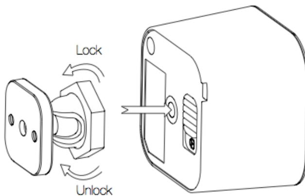
3. The Back-Mount Arm may be locked at various angles by turning the Friction Lock clockwise and counter-clockwise to respectively tighten or loosen the angle of the arm. You can rotate the Friction Lock to change the measurement area of sensor.
