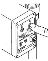
the system to activate. The valve will remain closed until the unit is manually reset on the WaterCop® panel. After the plumbing problem is fixed, reset the WaterCop® by pressing "open valve" (green circle) on the face of the WaterCop®. Valve will open and green indicator will be lit. See illustration at left.
