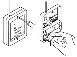
Follow suggestions found in the section titled "Placement of Flood Sensors" for recommendations where WaterHounds should be placed. Locate a wall near the area you choose to monitor. Avoid high traffic areas where cord or sensor could be stepped on or kicked. Mount transmitter at a convenient location on the wall, two to three feet above the floor. This will help avoid damage to the sensor and provide a strong signal. Use hook and loop fastener included with the unit.
