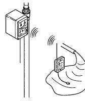
The flood sensors are a battery powered device enabling it to be located anywhere a leak is likely to occur, or where water might cause damage. The WaterCop® requires household electrical power (common 115 VAC, grounded outlet) and will not operate during a power outage.
