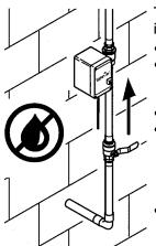
The shut-off valve must be installed indoors
