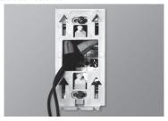
8. Align the little slots located on the top of the thermostat with those on the the mounting base and secure the thermostat to the mounting base. Note that you can also position the thermostat on the left or the right side of the junction box (see the illustrations below). Then, tighten the screw at the bottom of the unit.
