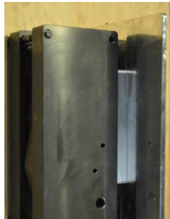
Figure 4.6 Install the rear shelf jig to mill out the trigger hole through the lower
