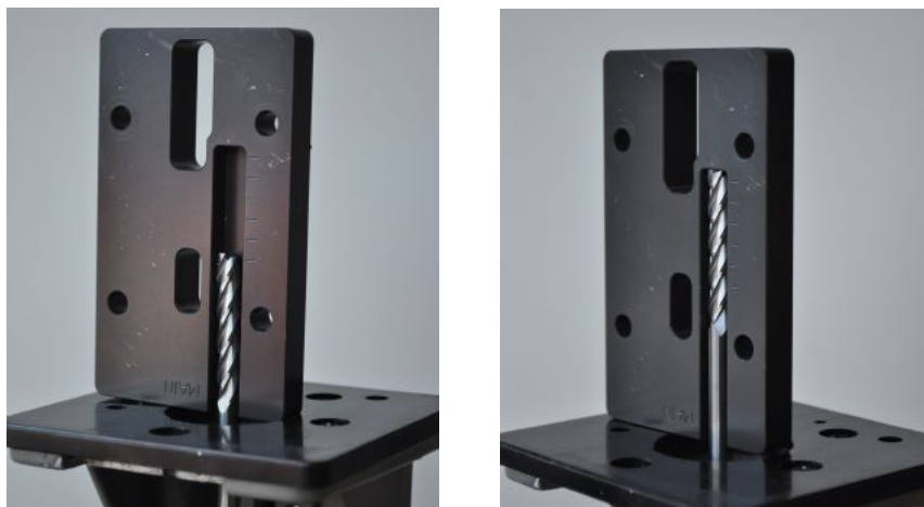
Figure 3.4: Left: End-mill set to the 1 st hash mark to start the trigger pocket, Right: End-mill set to the final depth resulting in a finished 1.249" deep trigger pocket
