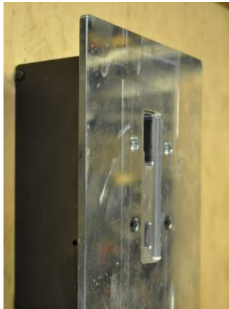
Figure 4.6 Install the rear shelf jig to mill out the trigger hole through the lower
