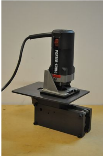
Step 4a: Mill out the rear shelf
