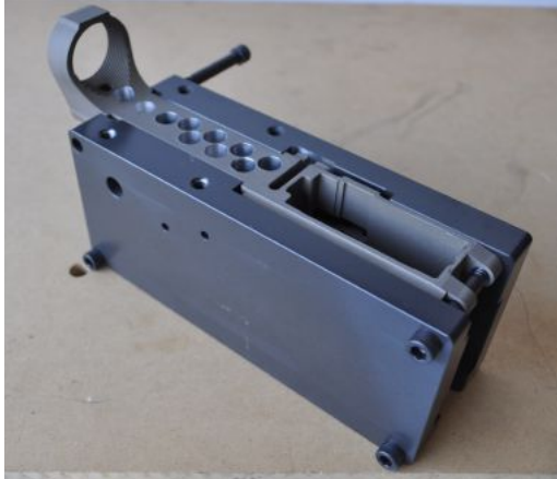
Figure 2.7: Remove the screw closest to the buffer tube – photo shows it removed and inserted into the other side for clarity
