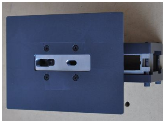
Figure 4.1: Trigger pocket orientation shown the "island feature" and proper orientation (Silver parts are used for clarify, all jig parts are the same color)
