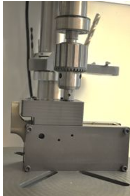
Figure 2.5 (left): Hand-drill at proper depth when the drill stop just touches the drill template Figure 2.6 (right): Drill-press at proper depth when the drill stop just touches the drill template
