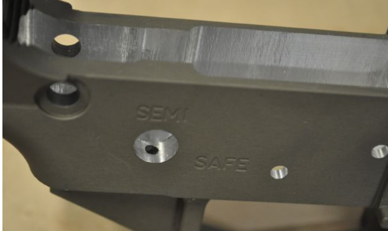
Figure 6.1: Difficult to clear burr in safety selector hole
