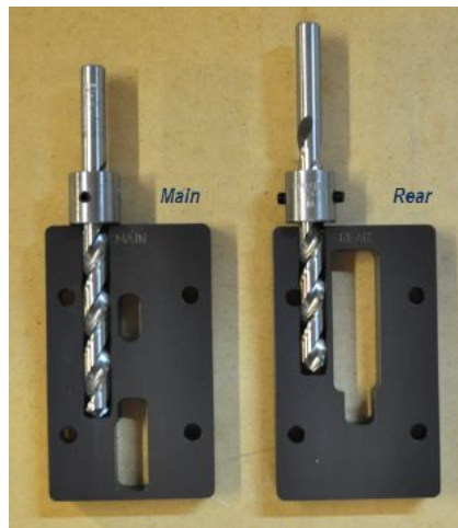
Figure 2.4 (left): Depth gauge used to set the drill bit for a finished depth of 1.249” (Main) or 0.630” (Rear) in the lower receiver
