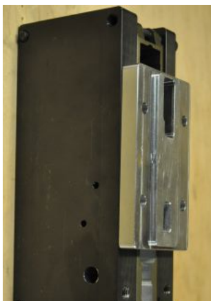
Figure 4.6 Install the rear shelf jig to mill out the trigger hole through the lower
