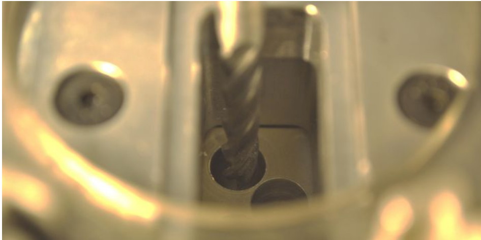
Figure 3.5: Starting with the end-mill inside of a drilled hole not touching the sides (photo is with a full sized router not a laminate router)
