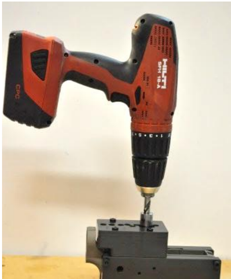
Figure 2.5 (left): Hand-drill at proper depth when the drill stop just touches the drill template Figure 2.6 (right): Drill-press at proper depth when the drill stop just touches the drill template
