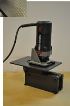
Step 4b: Mill out the trigger slot
