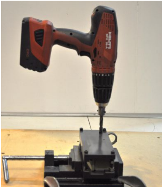
Figure 5.1 (left): Hand-drill used to drill trigger and safety selector holes
