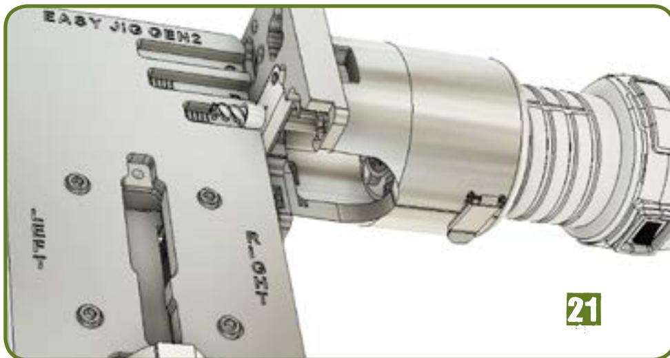
Press the router attachment plate flush against the right side of the jig with the bushing fully inserted into slot "A" (Fig. 21). Adjust the router depth so the tip of the end mill is on the first hash mark (Fig. 22). Tighten the depth adjustment on the router and insert the end mill into the 21/64" pilot hole (Fig. 23). Orient the router so you are standing behind the jig closest to the buffer screw.
