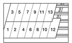
Apply sheet #1 in the lower corner. Apply #2 next to and sidelapping over #1. Fasten sheets at the purlins, taking care to keep them in alignment at the top and bottom edges and at the side laps. Do not fasten the unlapped edges. Apply #3 above and end-lapping over #1 and the top corner of #2.
