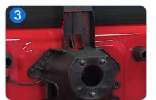
Expose the wiring harness as the figure showed.
