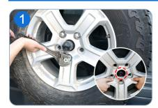
Remove the third spare tire (Note: Be careful not to damage the camera in the middle.)
