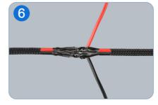
Glue all the wire harnesses with tape, then install the spare tire back on the vehicle, the installation is complete.
