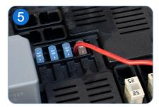
Connect the red wire ( RGB ) to the ACC or the wire of turn signal light (All fuses over 5A can be used. Note:Please use an extension cord if connect the wire to ACC)
