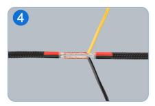
Cut the wire harness and reveal the wire cores. Connect the yellow wire of the spare tire light to the red wire of the original high brake light.
