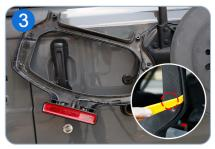
Use a plastic screwdriver to separate the plastic plate of the high brake light.
