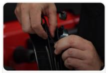
Plug the factory 3rd brake light in to the brake light ring harness, Plug the brake light ring into the factory harness
