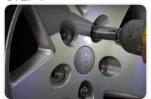
Remove your spare tire using a 19mm socket.
