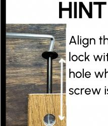
Align the cam lock with the hole where the screw is inserted
