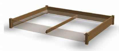
Attach the other side rail using a cam lock and screw in each hole. (4x)
