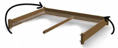
Insert the center support rail using 2 short screws.
